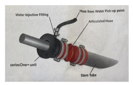
Later Shrimper 19s and all Shrimper 21s are fitted with a more sophisticated 'Tides-Marine' propeller shaft seal. There is no more screwing down on the grease cap to force waterproof grease into the earlier system. Now the boats are equipped with a 'fit and forget' rubber collar which is lubricated by a constant stream of water from the engine cooling system, and is not affected by minor misalignment of the shaft so should provide a very good seal for longer.
