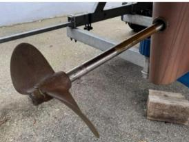
The important next step is to clean the complete propeller shaft. I used wire wool to get off all tiny barnacles and marine growth.
