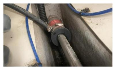
Access to the seal is not easy and the cockpit floor will need to come out. The photo shows the view looking back at the seal on a 21 with the floor removed. Note the lubricating water pipe from the engine. (The black corrugated tube is for the bilge pump).
