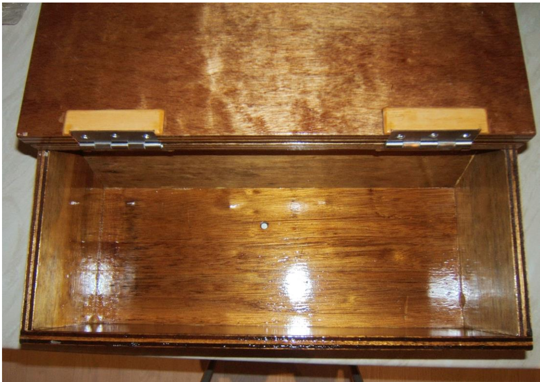
Inside showing wooden extensions at the hinges to allow adequate thickness for the screws
