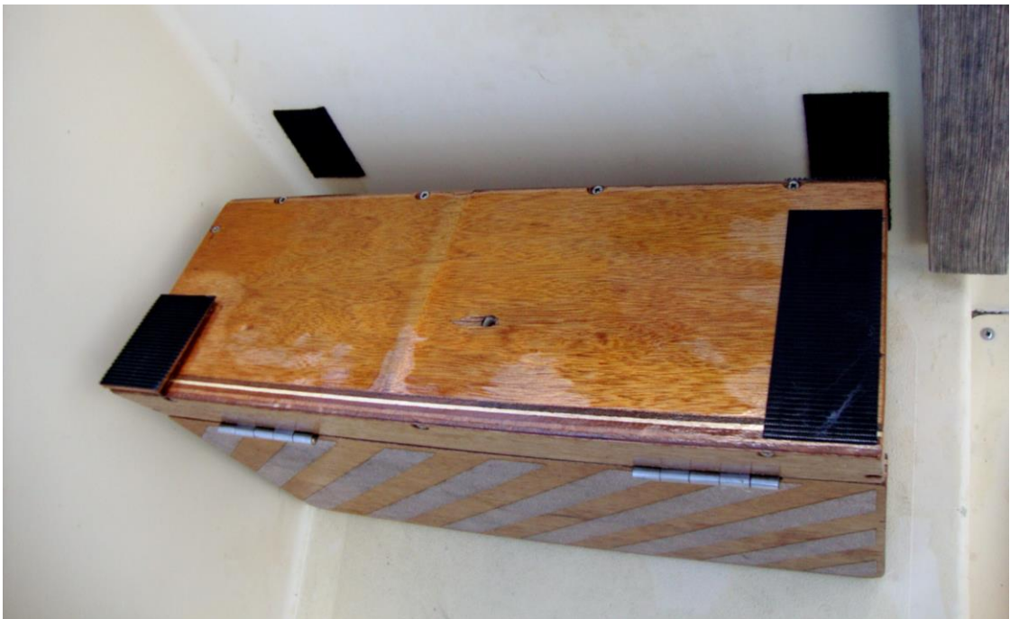
Box tipped aft to show the Velcro attachment
