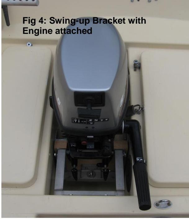
**Fig 4: Swing-up Bracket with Engine attached**
