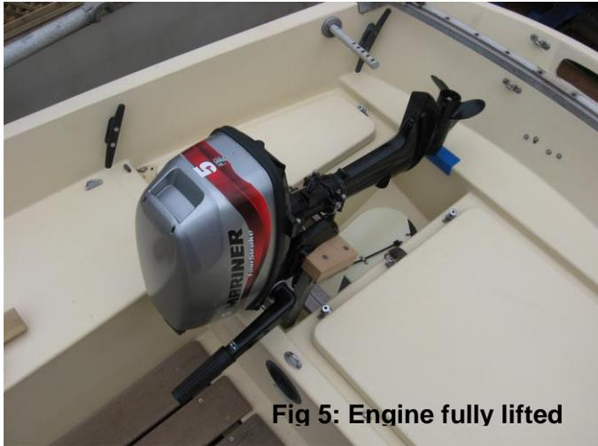
**Fig 5: Engine fully lifted**
