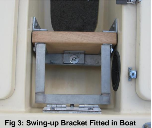
**Fig 3: Swing-up Bracket Fitted in Boat**
