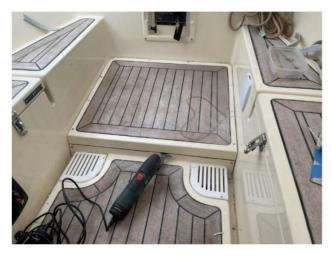
The next step is to remove all the screws holding down the floor, and then carefully go around the edge with a sharp knife to try to separate the white silicone mastic seal.
