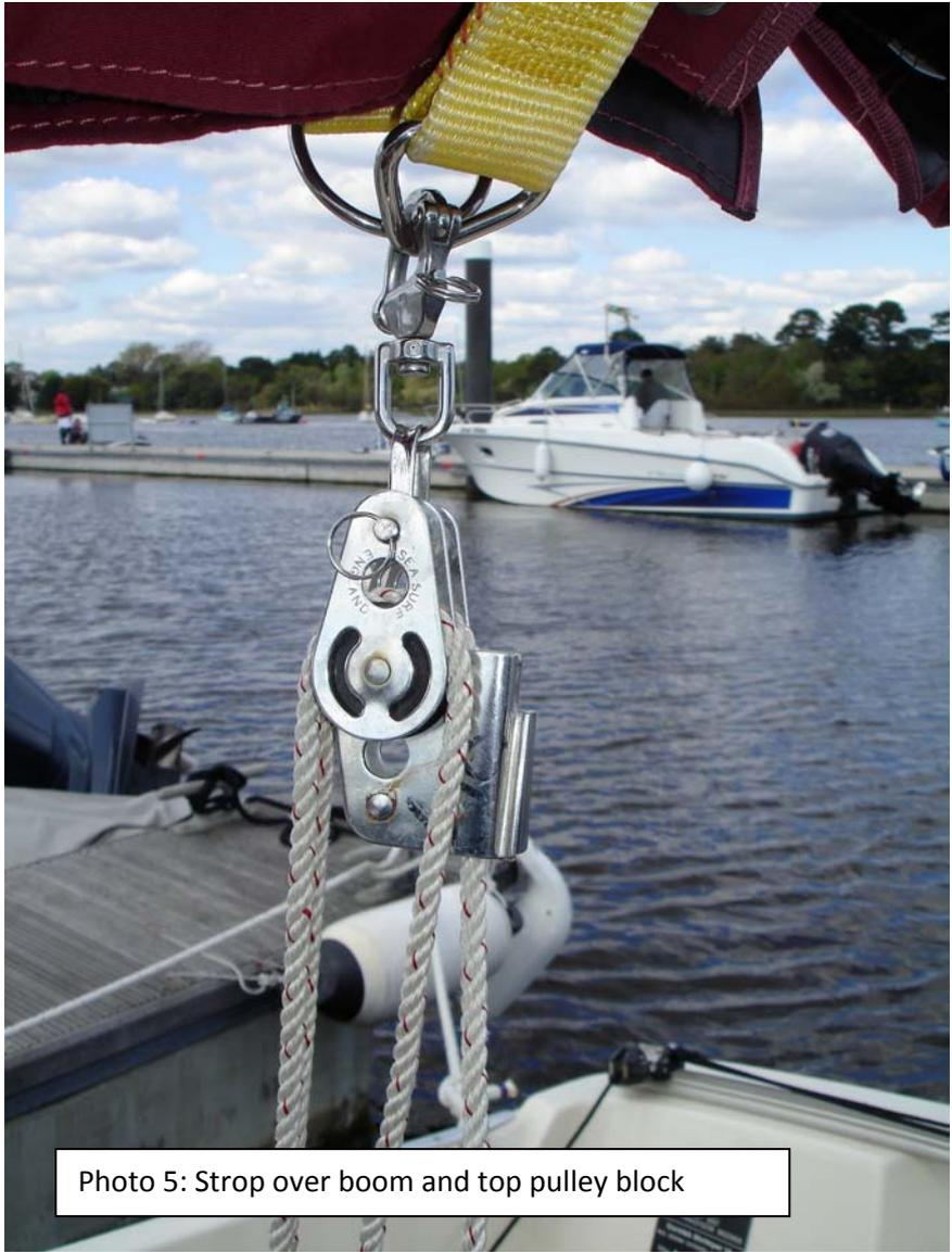
Photo 5: Strop over boom and top pulley block
