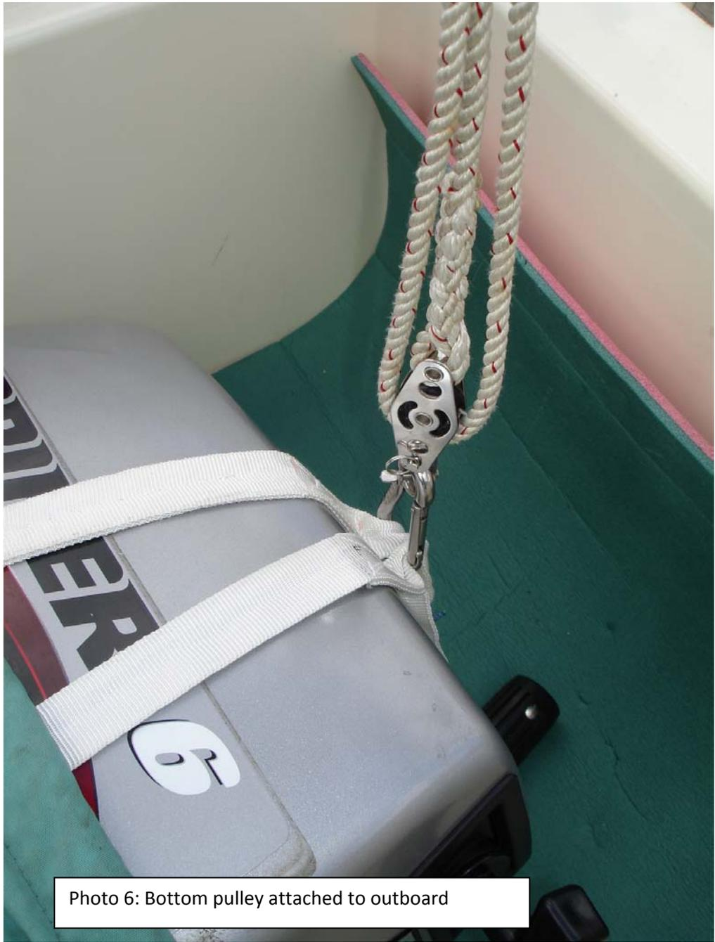
Photo 6: Bottom pulley attached to outboard
