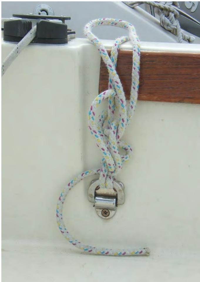
pivot bar of the D ring to be more square than round, which caused it to jam when lifted and rattle when folded down. A morning's work with a fine file produced cylindrical pivot bars, but the rings then rattled more than ever. The cure was a couple of turns of self-amalgamating rubber tape wound onto the bar, which had the additional benefit of holding the rings horizontal when lifted, making it easier to reeve the fender line.
