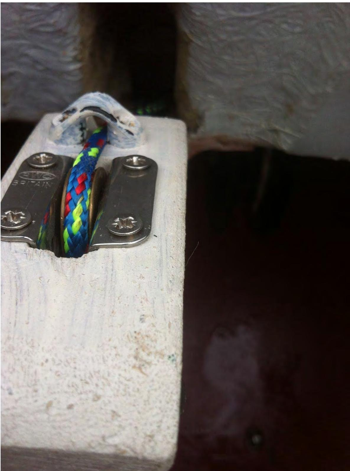
Figure 10 Close up of sheave mounting (painted)
