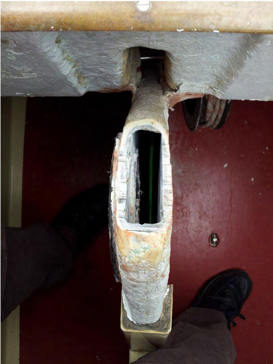
Fig 2 Keel box with top removed
