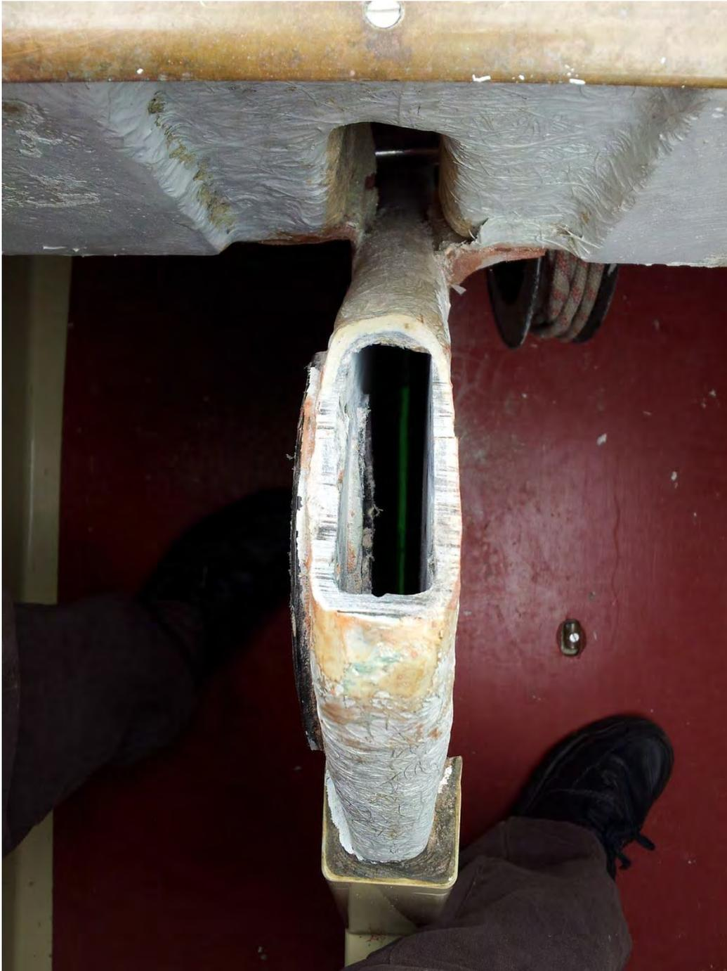
Fig 2 Keel box with top removed
