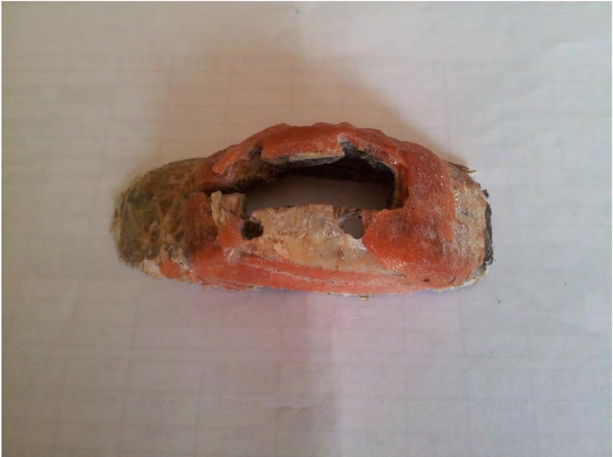
Fig 1 Original Sheave Mounting
