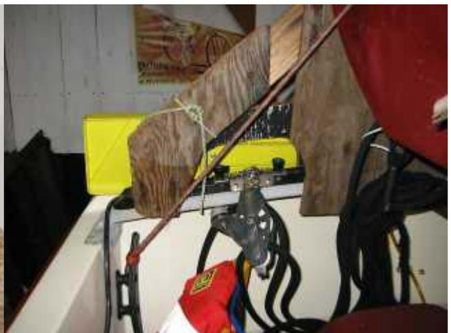
Pull the jib sheets in tight, close up the cabin, fasten lighting board and cable, and strap the boat down to the trailer.
