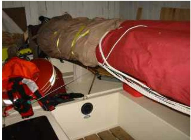
Fasten the Boom, Gaff and Mast to the support with an elastic shock cord over the top from cleat to cleat.
