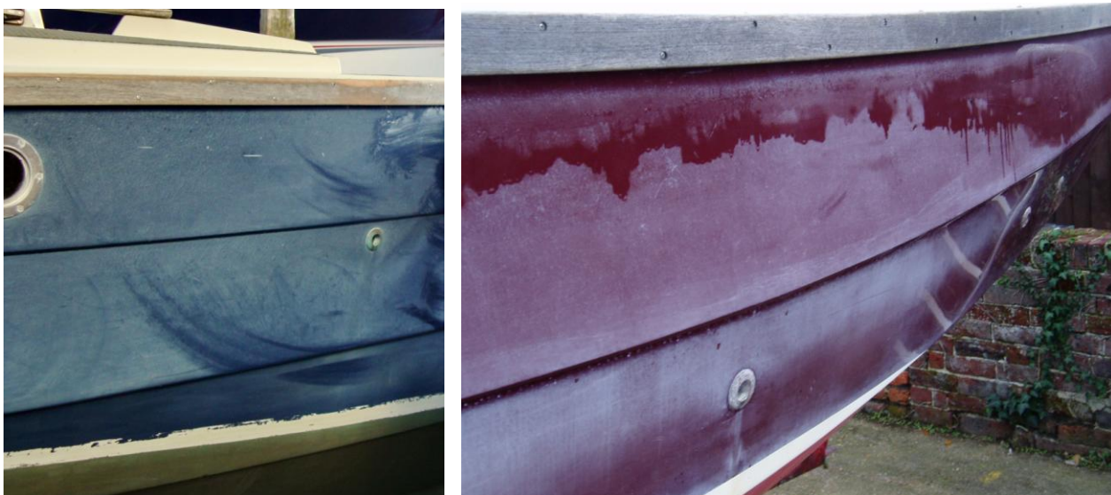
Hulls requiring Deep Cut
