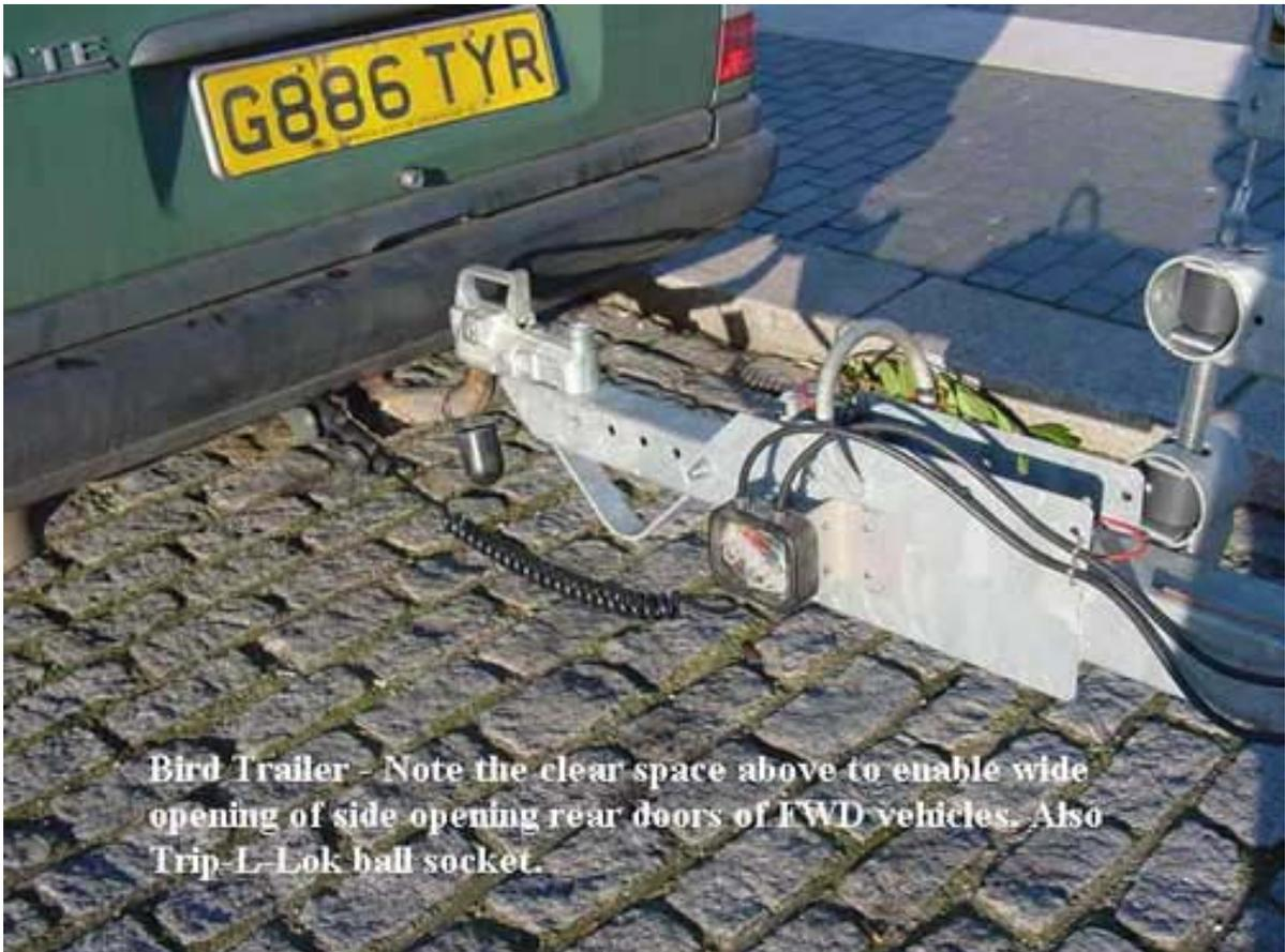
**Bird Trailer - Note the clear space above to enable wide opening of side opening rear doors of FWD vehicles. Also Trip-L-Lok ball socket.**
