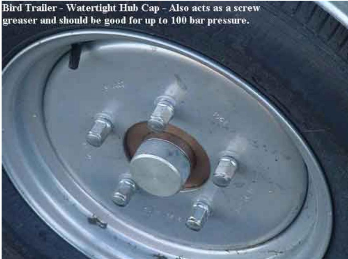
Bird Trailer - Watertight Hub Cap - Also acts as a screw greaser and should be good for up to 100 bar pressure.
