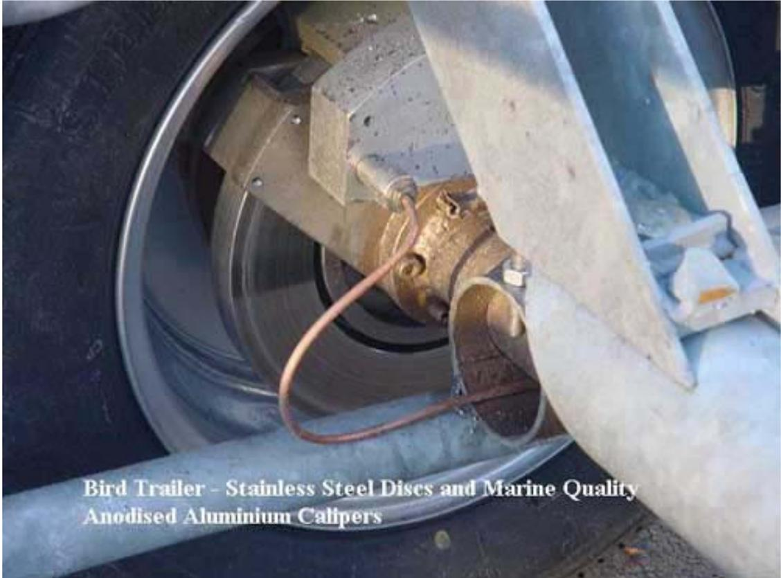
Bird Trailer - Stainless Steel Discs and Marine Quality Anodised Aluminium Callipers
