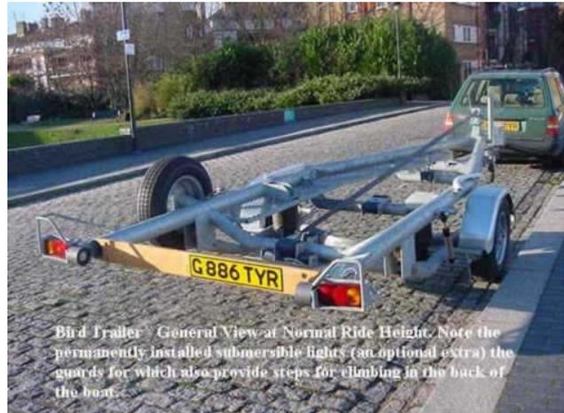
Bird Trailer - General View at Normal Ride Height. Note the permanently installed submersible lights (an optional extra) the guards for which also provide steps for climbing in the back of the boat.
