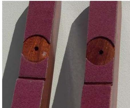
The moment of truth had arrived and the legs were attached. We were delighted when they fitted perfectly, looked very handsome, in keeping and in proportion with the hull and with the Shrimper philosophy. Final measurements were taken with the legs in place marking the line of the keel against each leg then cut off the excess plus one inch to ensure that the legs would take the ground after the keel.
