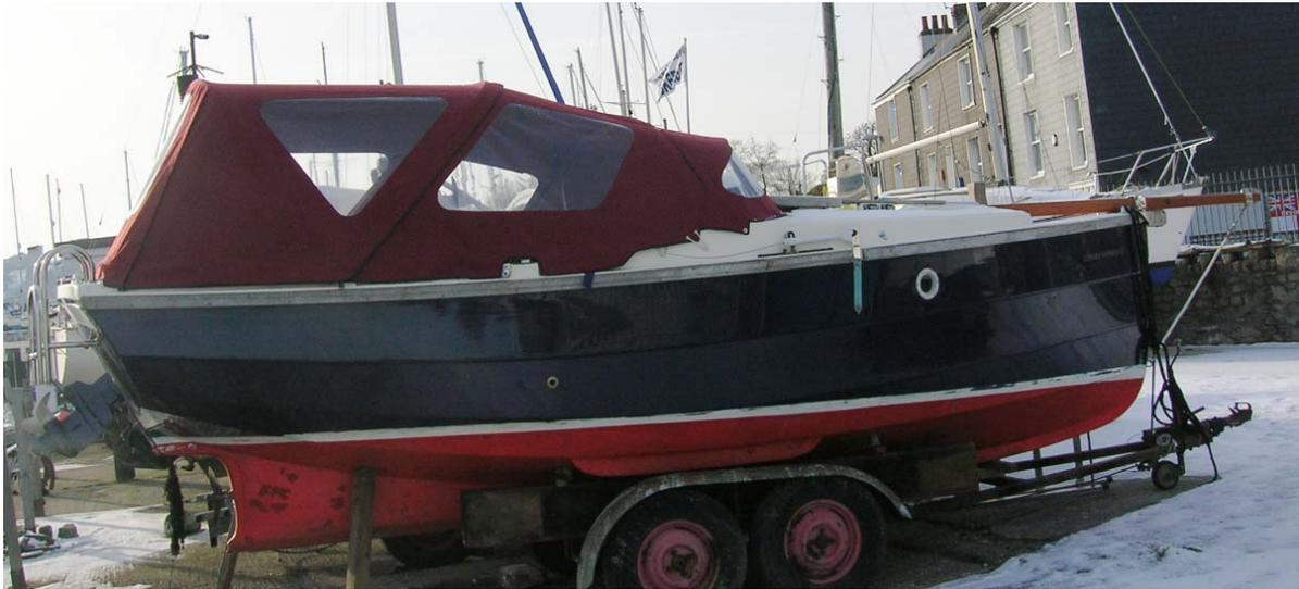
This tent was made in collaboration with a Plymouth cover maker. I wanted to avoid the closed-in feeling and condensation problems of a conventional tent with its exposed hook fittings on the topsides.
