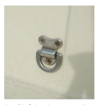
pivot bar of the D ring to be more square than round, which caused it to jam when lifted and rattle when folded down. A morning's work with a fine file produced cylindrical pivot bars, but the rings then rattled more than ever. The cure was a couple of turns of self-amalgamating rubber tape wound onto the bar, which had the additional benefit of holding the rings horizontal when lifted, making it easier to reeve the fender line.
