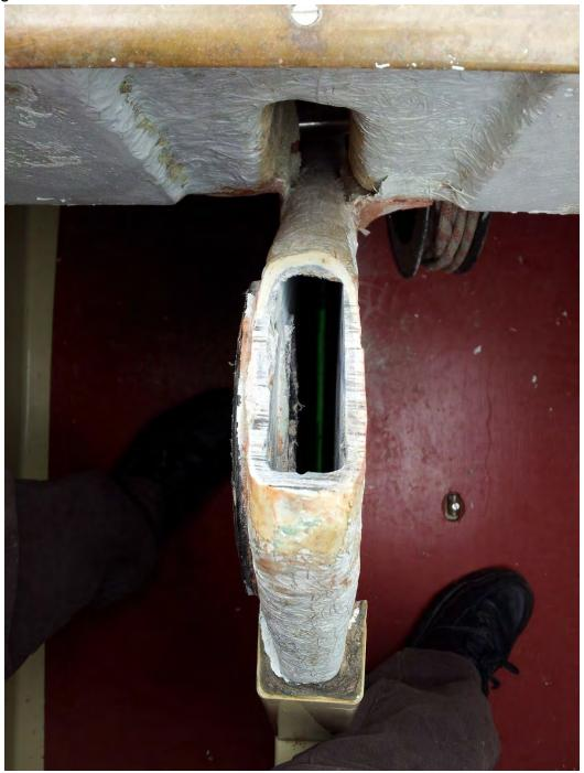
Fig 2 Keel box with top removed
