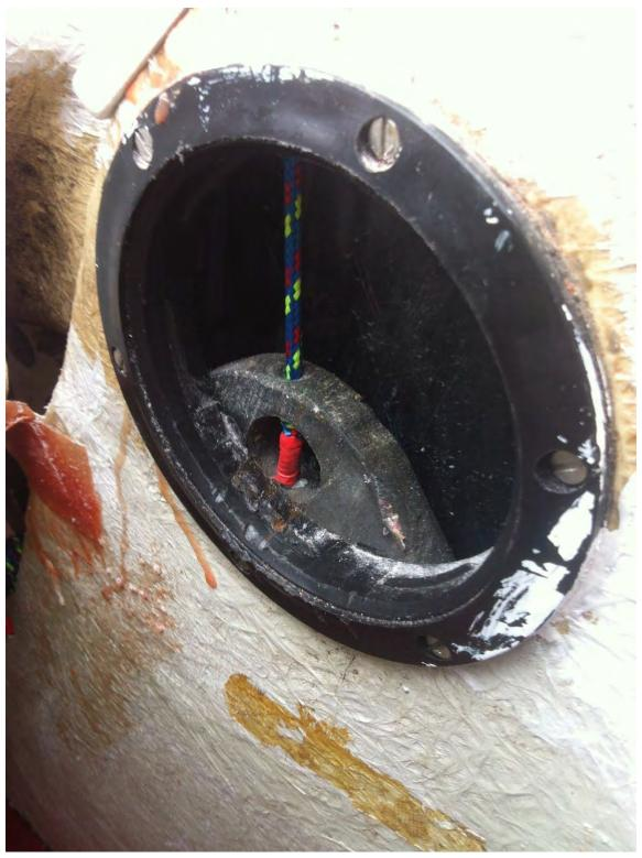
Figure 9 4 mm Dyneema threaded through
